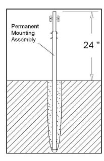
It is suggested that the antenna be tried in an area using the permanent mounting assembly in a hole in the ground before concreting, in case the antenna needs to be moved later. Once you are sure of the location for the antenna, the Permanent Mounting Assembly can be concreted into place, if desired.
